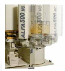
MITER SHEAR UNIT Flar bar cuts (-45  $^{\circ}$  to +45  $^{\circ}$ )
