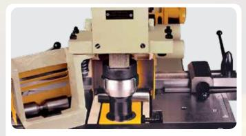
Punching equipment up to  $\varnothing$  36 x 8 mm. in thickness
