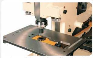
Goose neck die-holder for punching of  $\sqcup$  and  $\exists$ sections on legs and webs. Quick tool change.
