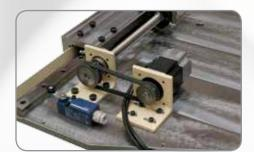
Basic Semipaxy Version detailing servo drive-spindle-encoder assembly
