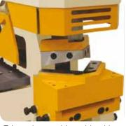
Triangular notching with table. Bendicrop 85SD This station can also be used for tube notching.
